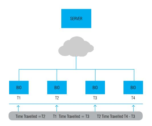
This data is used for travel time calculations as well as determining travel patterns around an urban environment. The server also uses these data collectors to send information and traffic conditions to road users that have the associated application installed on their personal phone or tablet device. This allows the server to issue public broadcasts to the road users using our BIO device to send warnings that can convert text to speech to inform the driver in real time.
